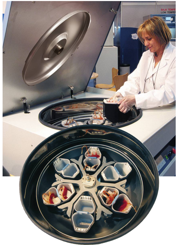
Image showing the rotor and double buckets for quad and triple blood bags of 500 and 800 ml.
