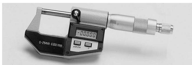
**PALMER MICROMETER WITH DIGITAL DISPLAY DIN 862**
