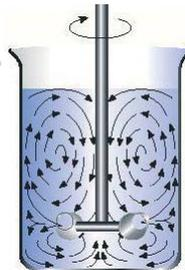
**Dynamic radial flow**, diagram showing the principal of agitation through a cone within the liquid. Representative of the Visco-Jet®. Rotors. Excellent results for minimum power consumption.
